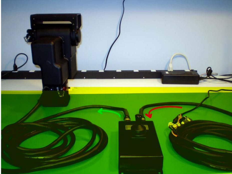
Figure 1 Setup Overview (arrows mark power flow)
